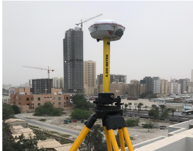
Fig.6 KUWT station data collecting device
