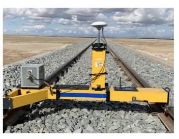
position of the railway track. The efficiency of track measurement was improved by dozens of times, and the risk of safe production of railway online operations was greatly reduced.
